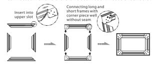
**Note:** after assembly of frames, please pat slightly position A and B, please check below. If there is seam appearing, please loosen screws on corner piece for adjustment until it is seamless before tight the screws again.
