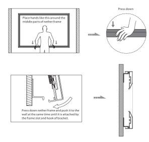
If need to uninstall screen, by following the same way as above, place hands on the middle of nether frames, press frame down and pull it outward until it is unattached from nether mounting bracket. Lift it to uninstall from upper mounting bracket. Please check below:
